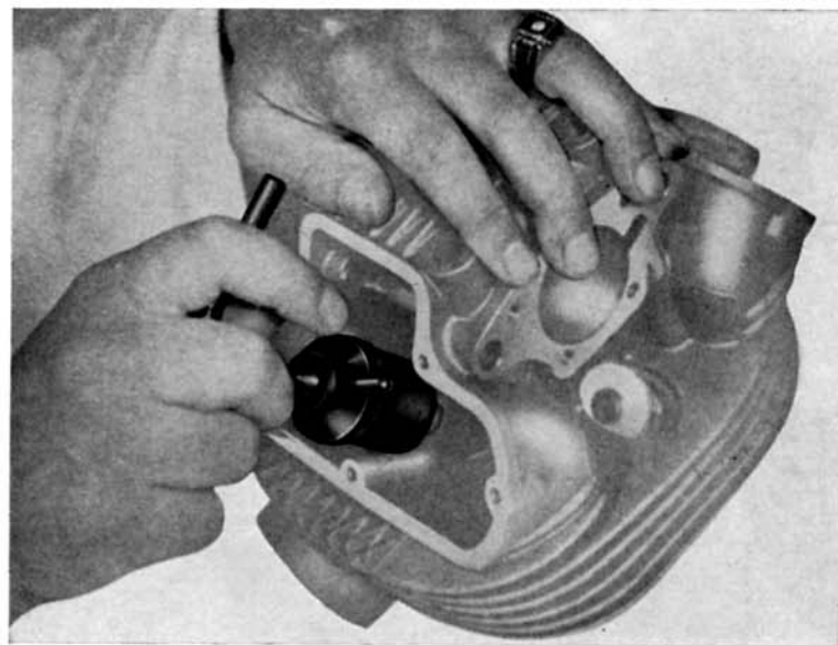
8 - Clamp for lapping the valve seats
